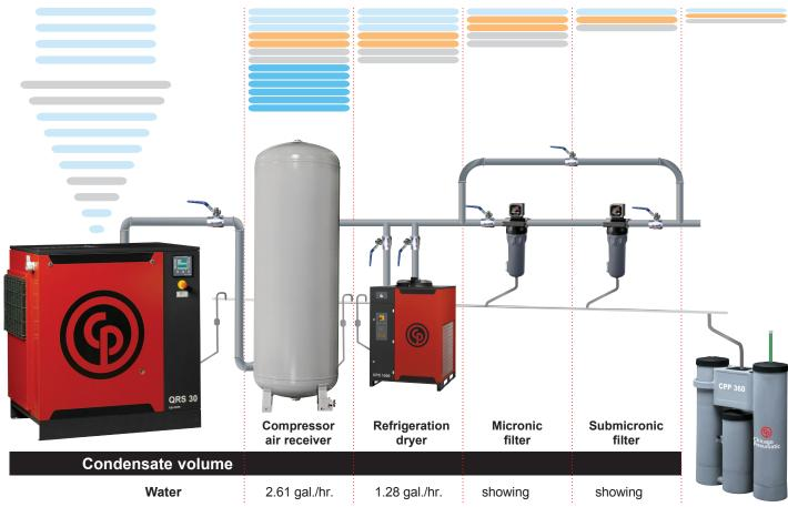
This drawing illustrates that during the air treatment process, 4.07 gallons of water per hour, plus dust, and 3,159 mg/hr of oil are produced.
