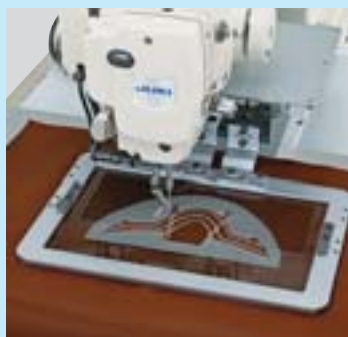
AMS-221EN-HS2516 Shape-tacking of a toe box
